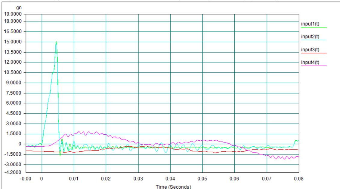
Figure 23: A typical terminal saw tooth shock plot transversal (X) 7,6g @ 11ms
