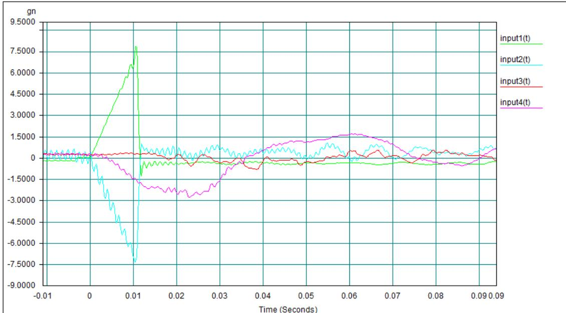
Figure 24: A typical terminal saw tooth shock plot transversal (X) 15,2g @ 5ms
