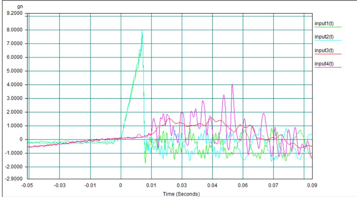
Figure 20: A typical terminal saw tooth shock plot vertical (Z) 15,2g @ 5ms
