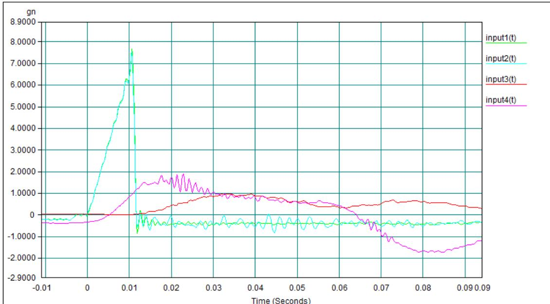
Figure 22: A typical terminal saw tooth shock plot longitudinal (Y) 15,2g @ 5ms
