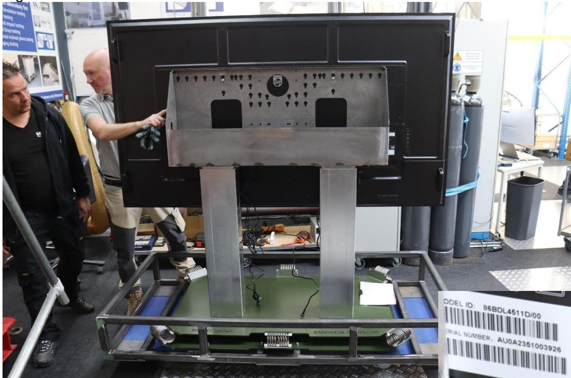
Figure 3: Test direction vertical (Z) and accelerometer location
