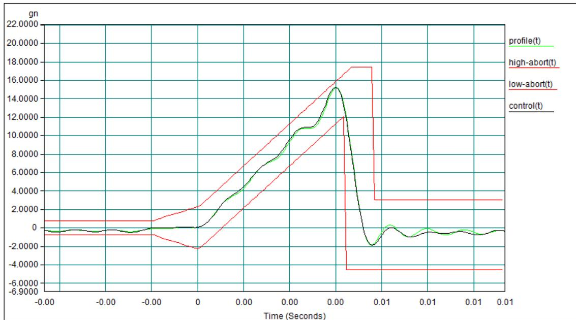
Figure 19: A typical terminal saw tooth shock plot vertical (Z) 7,6g @ 11ms
