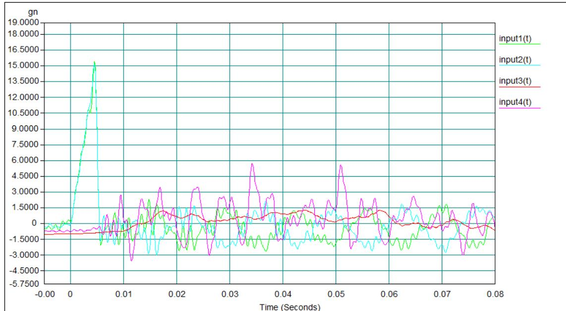
Figure 21: A typical terminal saw tooth shock plot longitudinal (Y) 7,6g @ 11ms
