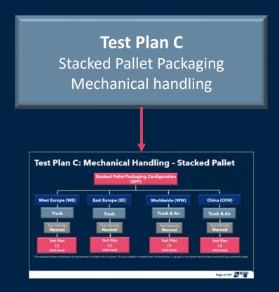
Within this document the test-procedure for a single-packaging and a (combination) of pallet-packaging's will be determined and clarified. Section 8 of the ASTM D 4169 describes the complete procedure to achieve a uniform basis of evaluating, in a laboratory, the ability of shipping units to withstand the distribution environment.
